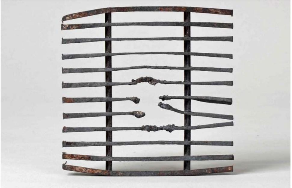
Above: A melted stainless steel grate from Jim Macdonald's heavily used 'Sweet Pea' locomotive gave rise to debate as to locomotive firing and draughting as well as to grate types and construction
