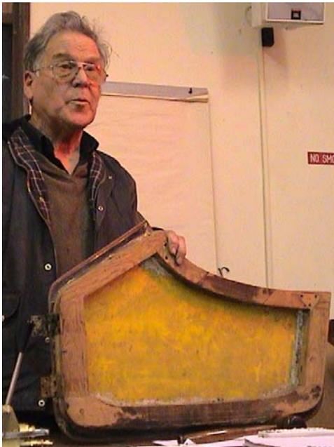
Mike Hodgson (left) has made a replacement car door for his Morgan, a two seater open topped sports car. The original door had rotting wood and rusty metal with holes right through. The wood joints used in the replacement door were made with Scarf joints. Mike drew sketches on
