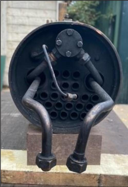
At the front end the superheater visually looks fit for purpose but a pressure test will be completed to prove the visual inspection is correct. The wet header showed no evidence of any past leaks.
