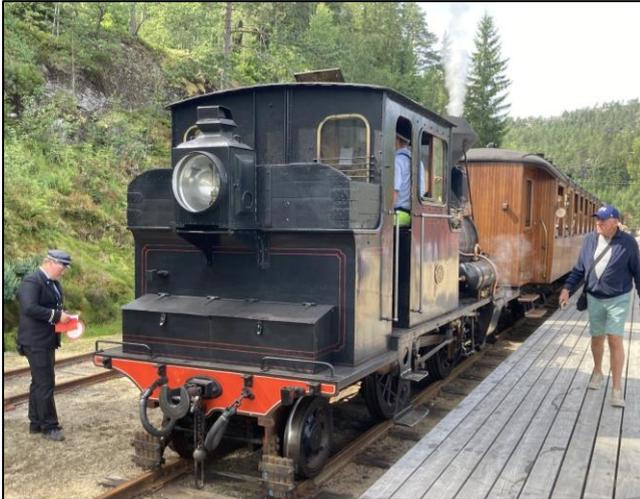
locomotives were rescued and have now been brought back into use. The original locos, 2-4-2T, were supplied by Dubs and we had locomotive no 5, a copy of the earlier locos, which was built in Norway.
