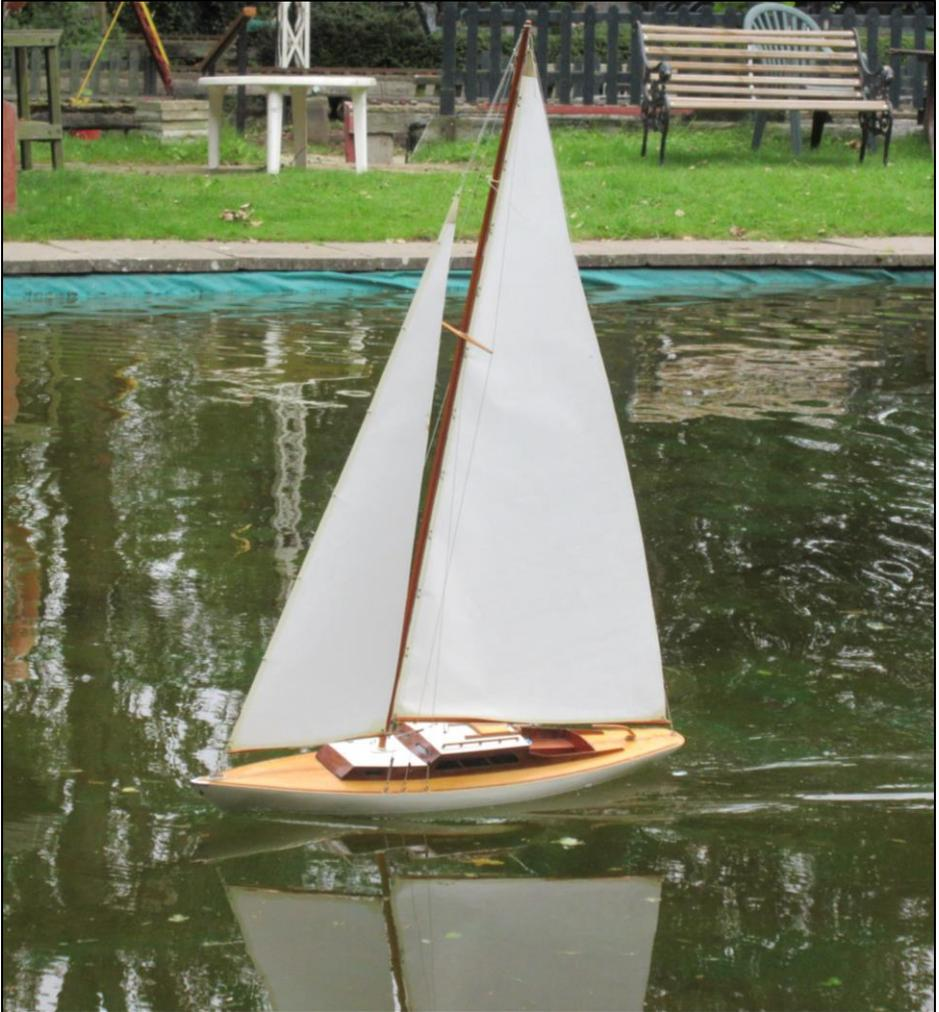
She took a while to assemble and I made all the bowsies and wire hooks needed. The yacht runs on a single 4.8-volt high capacity NiMH battery and uses 2 channel radio control. She is a pleasure to sail and has got wet quite a few times.
