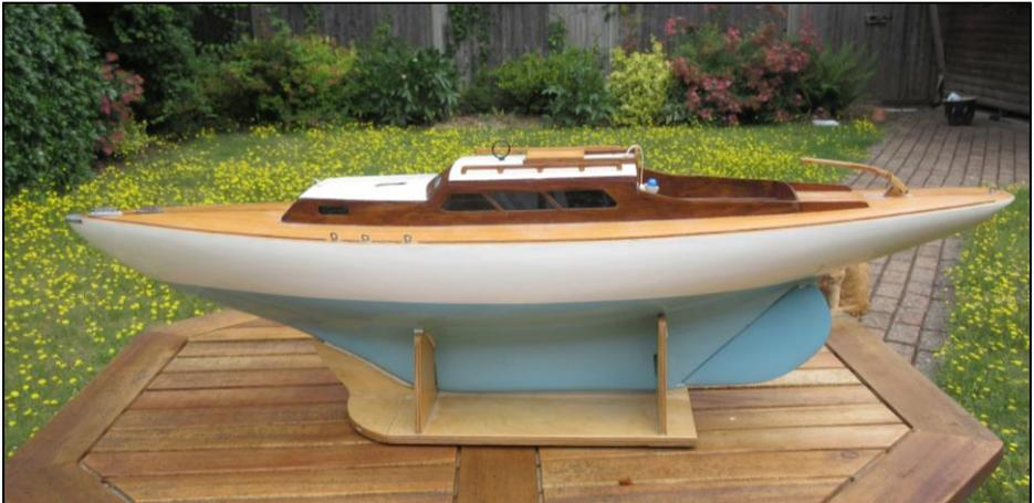
The rudder had to be made and you will notice it is not a straight up and down job. I make up my rudders using a ply frame and thin ply, when sanding to shape the various layers of ply show where the sanding has taken place, a bit like contours and it is easier to create an even shape.
