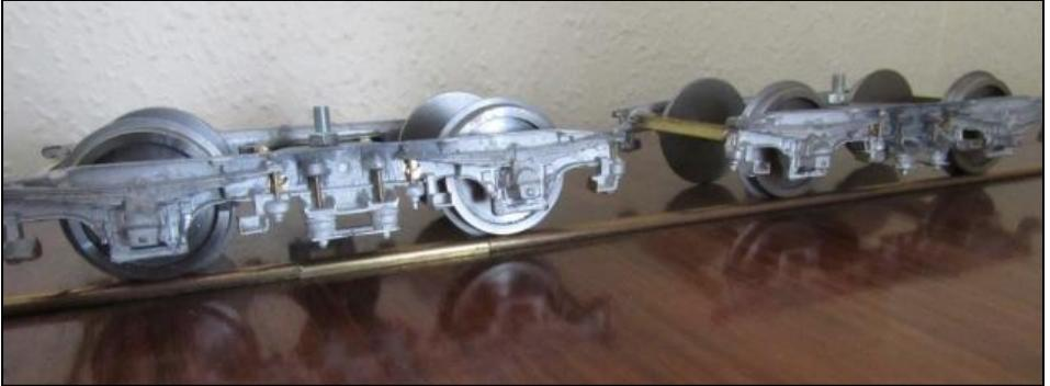
the supplied bits so I have just made them up as JVR type bogies with PTFE bearings and they seem to roll very well. There is an opportunity to add a few bits of detailing for the spring supports on the castings which you can see I have done with Brass rod.
