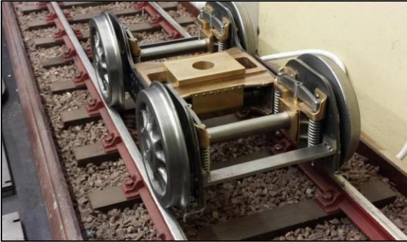
I later changed the way that the irons are bolted to the frames just to make things more practical. I haven't set the springs yet in this picture, it's probably best to do this once the loco is close to completion or at least after the boiler is sitting on its frames.
