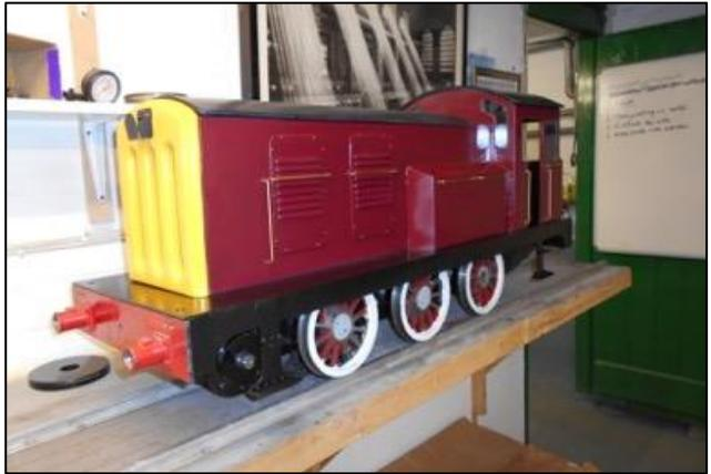
I bought 6 spoked wheels which needed lead balancing weights fabricated, easy so far! Next the couple rods, I spent a long time making them and was well chuffed when other proper model engineers complemented me on their appearance. I made a rolling road fitted coupling rods on one side everything worked perfect. Fitted the rods on the other side and everything ceased up solid! Quartering had never been a problem before but I just couldn't fix the problem.
