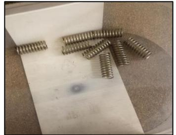
The next job was to make the spring pins, I decided to make these in two parts as done a number of times with similar parts to save time. The first part being the
