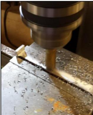
Once they had been tidied up a little, they both had their ends machined square until they were exactly 4" across, the picture then shows the rear stay being machined down in thickness to the 2 mm shown on the drawings although I left the ends a little thicker for more strength.
