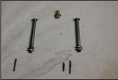
I added oil cups to the top of each spring yoke on either wing to directly feed these points
