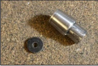
The picture shows a cut rubber disc along with the tool for doing it, note the hardened tip just visible.
