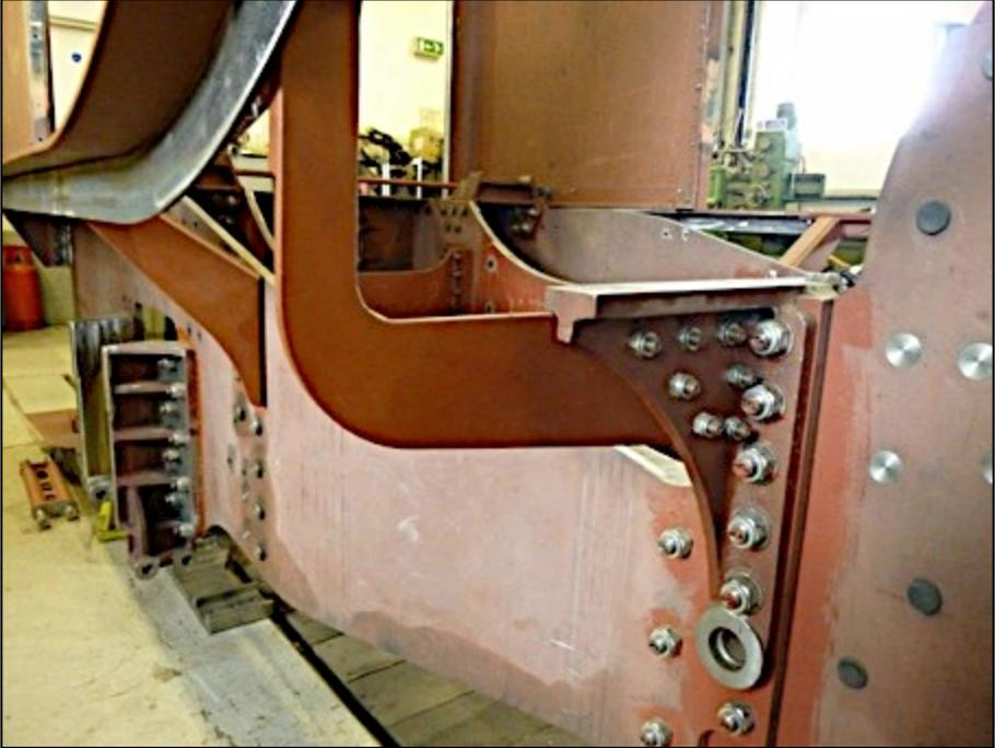
The two photos are of the new build construction of an LNER Gresley P2 2-8-2 locomotive in 12" to the foot, taking shape at the Hopetown Works, Darlington. Of particular importance is the smokebox being erected on the frames for the first time, being sponsored by the Gresley Society. Nice detail shot of the rear frames for anybody (i.e. me) building a Gresley engine with same style of foot plating, boiler and cab.
