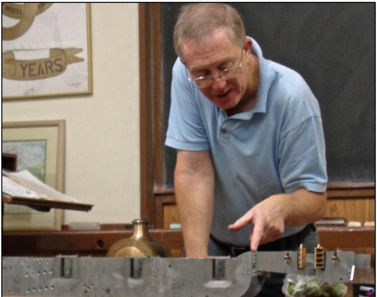
state of the art DRG to spot and drill the holes for the stretchers and horn blocks and then the good old hammer and vice to teach the curvy bits of frame how to behave. Forming a very fine embryo of a five-inch gauge locomotive which will no doubt take two members to lift onto the table at the next WIP.
