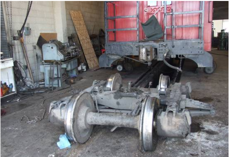
Bottom left: Engineers disassembling a bogie to repair a “hot box” suffered on the previous days service from Chama to Antonito. Above: The melted axle box white metal bearing. Below: The completed bogie. Photos: Les Dobbs
