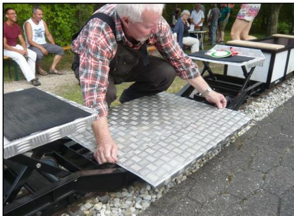
which was convertible into a disabled wheel chair carrying carriage, by the simple expedient of sliding the floor-plates apart, all engineered to a very fine standard.
