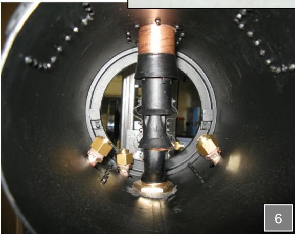
So, when the parallel chimney part is slid down from the top of the chimney onto the sliding joint the whole assembly becomes rigid. **(photo 6)**
