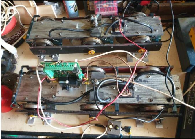
and gears a bit of a clean and some oil then with some temporary wiring gave both bogies a test run which went very well. As you can see there were plenty of wires in evidence but all will be sorted out and tucked away for the first run.
