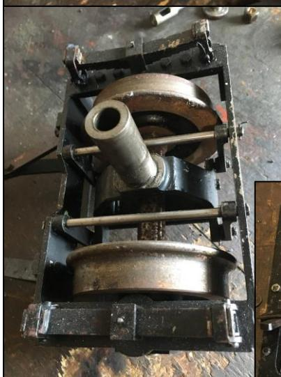
Leading and trailing bogies were also found to be in a similar condition and went through the same process of stripping cleaning and reassembly.
