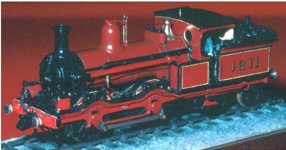
*Tim's 0-4-4 back tank. As used on the Midland suburban lines. Completed 1980, the model is less than 2 1/2in. long. Photo: Tim Watson*
