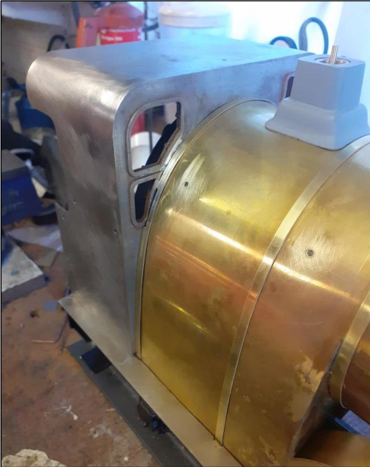
Then onto the cab, again laser cut. This comes in two parts, cab roof, sides and the cab front. The cab roof requires two bends in it to make the sides. The two pieces are then riveted together using 1/4" brass angle. I finally ran a bit of solder around the edge to fill any slight gaps.
