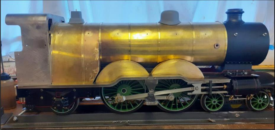
For the lagging I used 1.5mm thick ceramic fibre sheet which I found surprising easy to cut for the bushes for the dome and safety valve, simply place ceramic fibre sheet over the bush and run your finger around the edge of the bush and the hole is formed. To make the cladding I used a sheet of 26-gauge brass and thick paper to make the template. Boiler bands are made from 3/16" wide brass.
