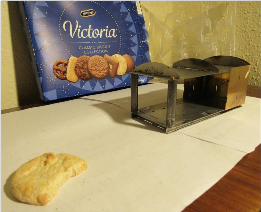
As you can see, I have made the main body structure from Steel plates, the upper and lower are actually the same plate, but the slots are only used in the top one for the curved roof supports while the groups of 4 holes are used for attaching the axle guards in the lower ones only. I am using bits of bar at the corners to give support to the rounded shape and also as strong support pillars for the upper
