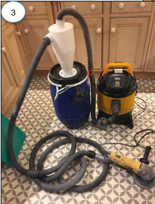
Now with the 3 components I started to assemble the revised cyclone: Drill a 67mm hole into the centre of the lid and 6 x 5 mm holes for the fixing roofing screws and nuts for attaching the cyclone to lid.
