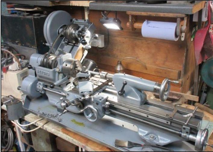
repair was the belt guard that had a crack to one corner I did try to MiG weld the aluminium casting but it really needs to be TiG welded alas I don't have a TiG welder?
