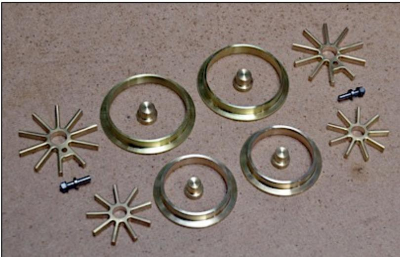
Wheels were fabricated from materials to hand, including a short length of thick walled brass tube for the driving wheel rims.
