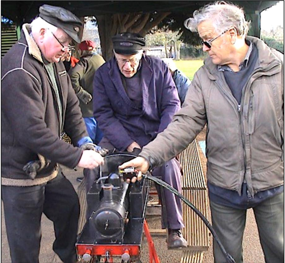
**Photo above.** Mike H on the water pump filling tanks with Jim operating the hand pump supplying the boiler with water. Mike F, the driver at this time, looking on in anticipation of a good run.
