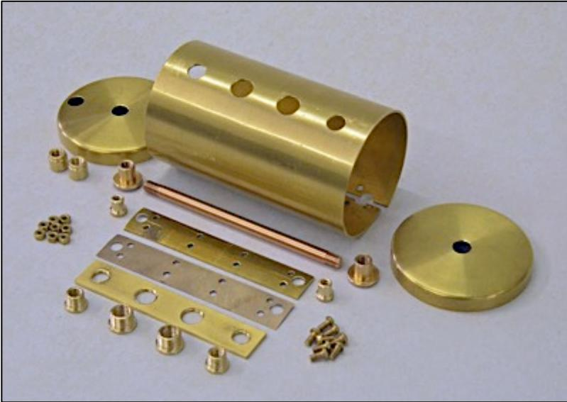
The boiler shell was rolled from brass sheet and fitted with a centre stay.
