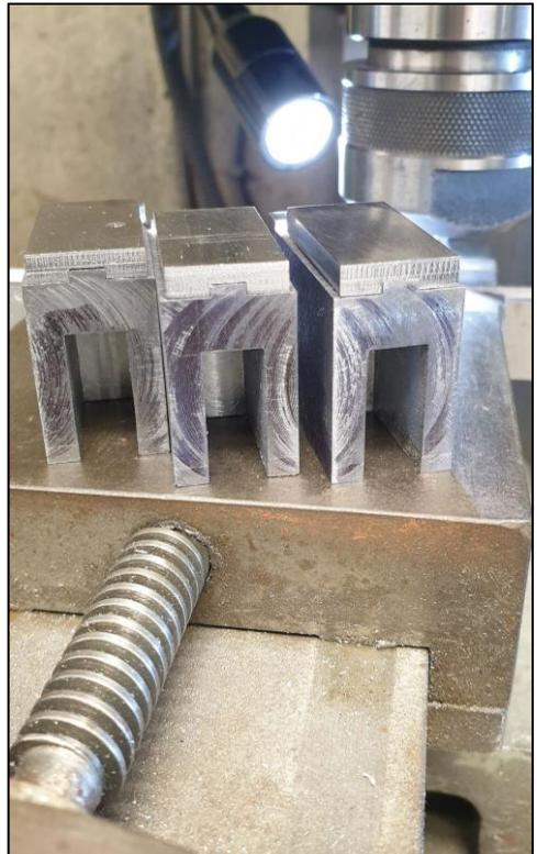
As well as trying to follow the prototype, I have also changed the design to suit what I think works best. One such change is in how the piston rod is secured in the crosshead. As drawn by Don the rod slides in the crosshead and is secured by a taper pin, others may go further and taper the rod as per full size.
