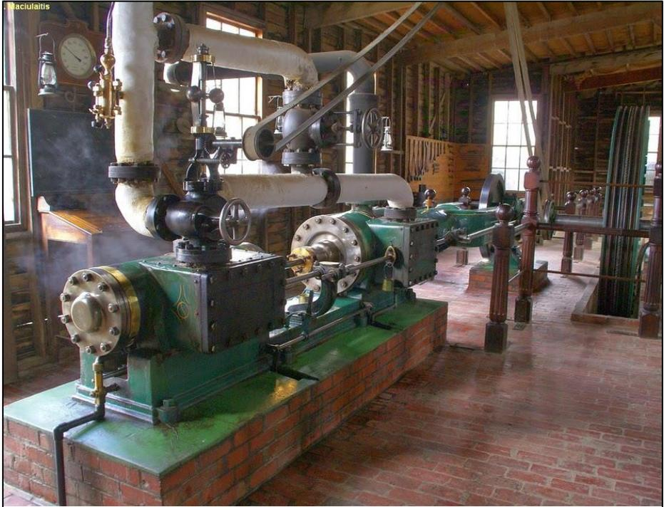
Still in full working order it became the subject of one of the clubs most prolific engine builder's latest project. The full-size 160 horsepower engine was built for the City of Ballarat in 1888 and supplied with a 110psi boiler by the Phoenix foundry for £800 to power a stone crusher at the local Alfreton quarry.
