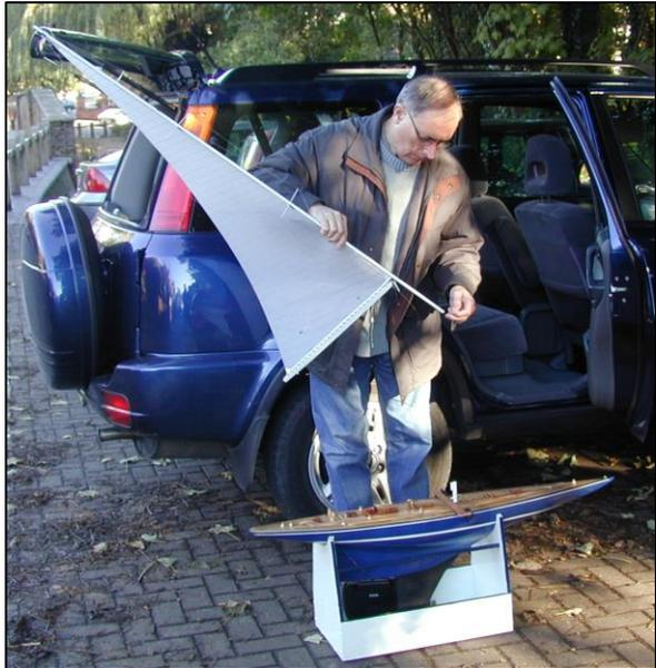
The Endeavour had a 'secret weapon' in the form of a 'quadrilateral' foresail, there was no way I could avoid it overlapping the jib so I just lived with it. The mast was a solid wood dowel and was also very heavy. I decided to fit an aluminium extruded purpose made mast, very light and a nice neat way to attach the sail.
