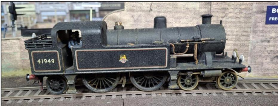
The remarkable thing about this model was not just the body shell but the printed chassis frames, bogies and, amazingly, the brass coupling, connecting and piston rods. Yes, that's right, printed brass! Other metals are printable too.
