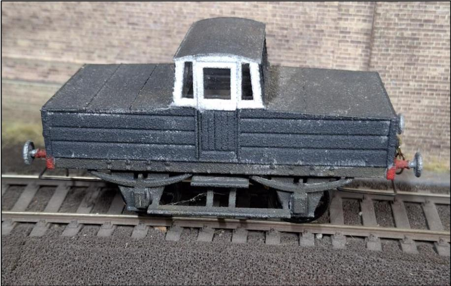
This often means that 3D Filament prints appear to have lines all over them and are less smooth than Resin. They do not require curing so can simply be snapped off the build area ready to paint. One advantage is that colour is determined by the filament that is being used and some printers can automatically swap between up to six colours. Personally, I find these colours to be too 'toy like' and the waste generated by the nozzle cleaning out between filament colours can quickly add up.
