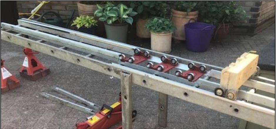
The real challenge was to work out how to get the loco positioned over the rollers without any manual lifting. As can be seen in the photos with a couple of bits of timber and some roller bearings for wheels I cobbled together a gadget to support the loco as it is moved into position over the rollers.
