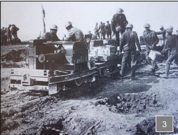
Photo 1 shows an armoured “open” cab loco and Photo 2 a fully enclosed armoured type. Photo 3 of a simplex is thought to be one of the earliest photos of one in action, and it shows one of the early 20HP locos used for evaluation.
