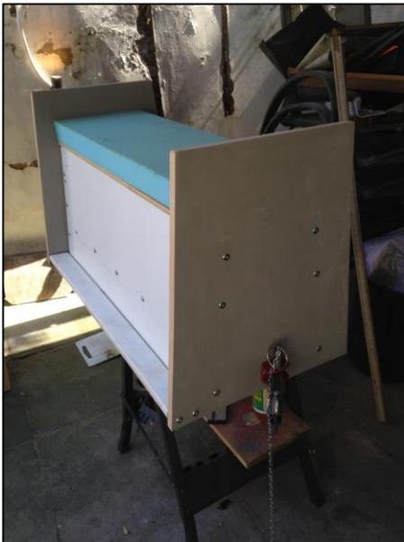
rectangles front and back and fitted it with some old dexion angle, but I did not like the way this was looking, it was too box like. So, I angled the sides 5 degrees. and sanded the ply ready for painting. The result wasn't very good so tried a different approach with some old beechwood cupboard doors which I cut to the thickness of the ply. I then machined a tongue and groove joint, applied adhesive and clamped the lot up. The finished appearance with a coat of acrylic paint was much better.
