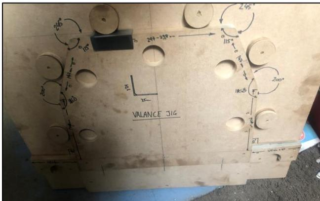
A jig has been made to help form/weld the valance end sections to the specification we gave but has since been altered to allow them to be made longer. The plan is for one "longer" end section to be made which can be attached to one of our existing carriages once the site reopens. It can then be
