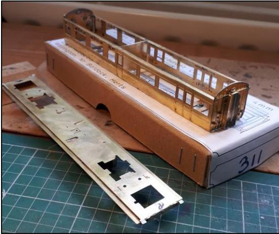
for which I use 3 different solders of various temperatures with fluxes to match. The trick to the soldering is to keep a very clean iron tip (not easy with the aggressive fluxes) and very clean components. It also helps to have various cunning methods to hold components in place when applying heat – especially the tiny pieces which have a habit of trying to stick to the tip of the iron rather than stay on the model. Fingers are useless (they burn) but
