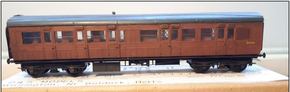
A key feature of the build of these and my restaurant car is fully compensated running gear which works on the “three-point suspension” principle meaning that all wheels are on the rails at all times.
