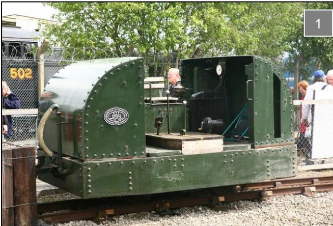
Soon they had developed their next version this used an improved 40HP Dorman engine and a 2-speed gearbox and it came in 3 versions the "open" this had armoured end plates with a canopy on adjustable pillars. The "protected" which was the same as the open but had armoured side doors and visors. And finally,
