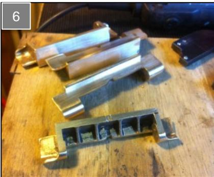
Finishing bogie horns and fitting to frames;
