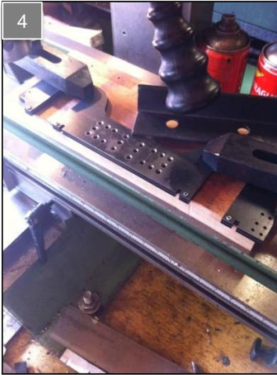
After bolting the frames together, they were turned around reset with DTI and clamped down. **(photo 4)** All holes were first drilled using a centre drill and followed with the correct size drill. The frames were then turned over for the other side to be countersunk.
