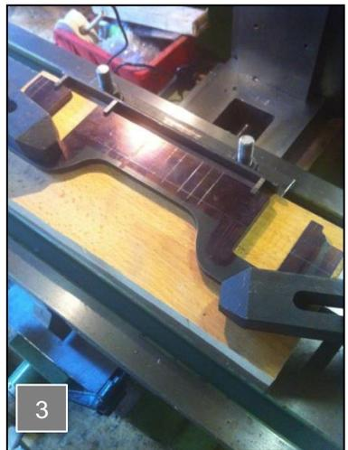
To get the frames bolted together, I decided to use the four horn stay holes to do this but needed to keep the frames in line first, this I did by cutting some pieces of steel of the correct thickness to fit in the stay slots and then lining these up against a steel right angle that had already been set square with a DTI. **Photo 3** shows this setup, I used a machined piece of English Oak to clamp the frames to for drilling.
