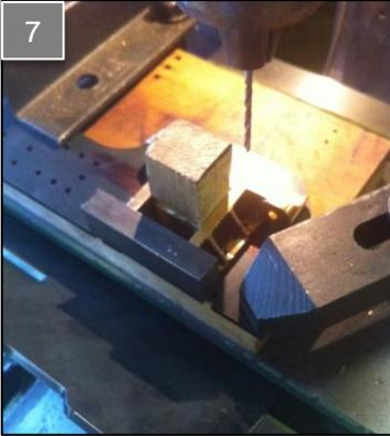
With the horn holes drilled next job was to turn the frames over and countersink them ready for the 5/64 rivets. **(photo 8)**
