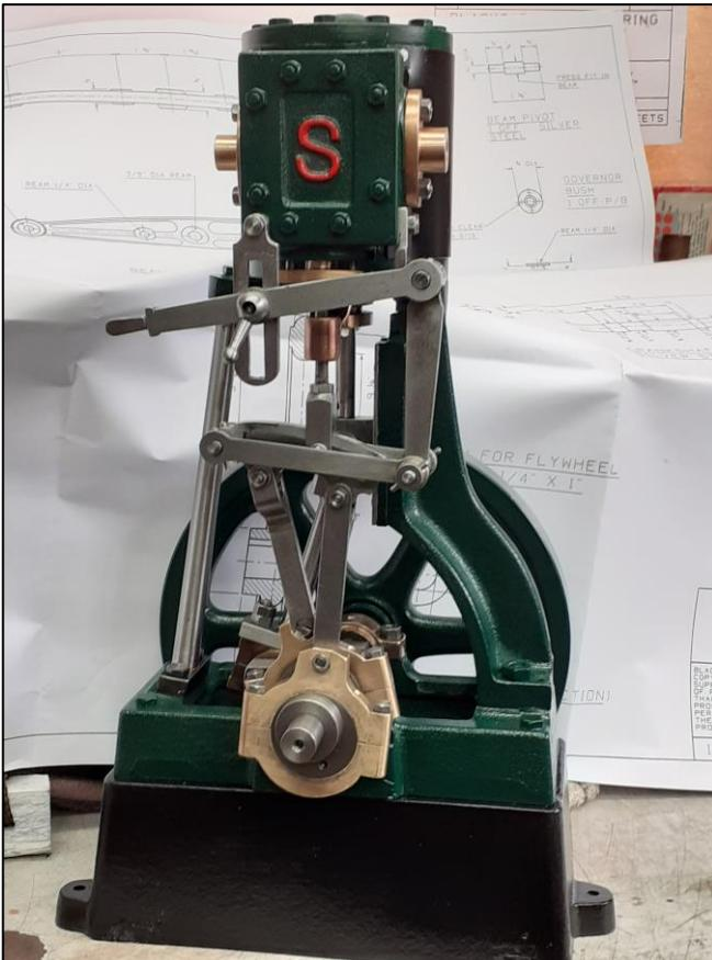
It has a 2" bore and stroke made in cast Iron.
