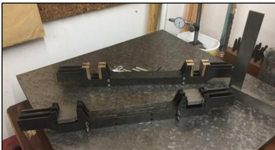
machine the horn guides to size. Very much like one would do so with the frames of a steam loco. Luckily, I have most of a box of slip gauges that I rescued from the stores scrap bin of a company I worked for. They were no longer suitable for the precision work they
