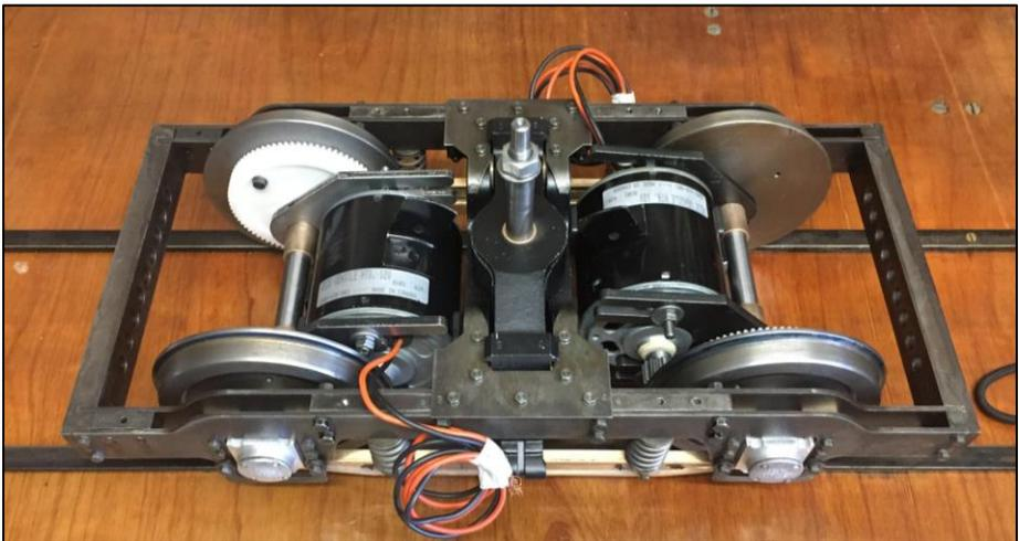
Later on in the final assembly I did have to come up with an alternative solution to that shown on the Dan Jeavons drawings of holding the motors in place to stop them rotating around the axle as all 4 motors hang on the axles and have to mesh with a gear attached to the relevant wheel.
