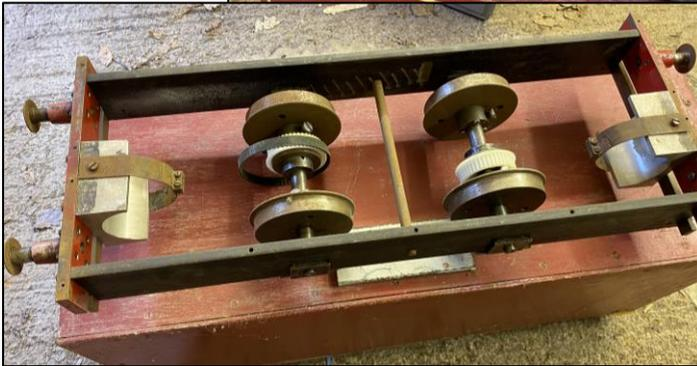
A 5 inch or 7¼ gauge diesel out line sprung chassis that has toothed belt pulleys, includes belts. motors and other bits. Body allows space for batteries but is a basic shunter outline.
