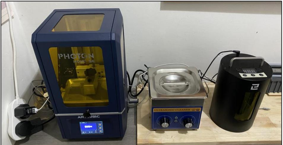
Photo 4; my most recent investment. A resin 3D printer along with an ultrasonic bath for cleaning excess resin and a curing station for setting the resin hard. This will be mostly for the axle boxes so detail is not compromised.
