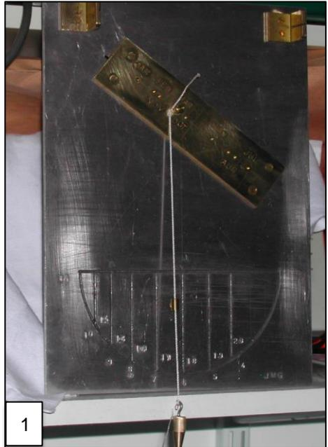
My first project was a “Capuchin Dial “made on a bit of scrap aluminium plate rescued from a cover of a piece of dead equipment. I spent a Christmas with a ruler and a scribe scratching each hour line into the plate. Numbers were created by using number punches. It was pretty crude, but I had to work with what few tools I had. I am not sure where the original dial is now, but here **(Picture 1)** is a
