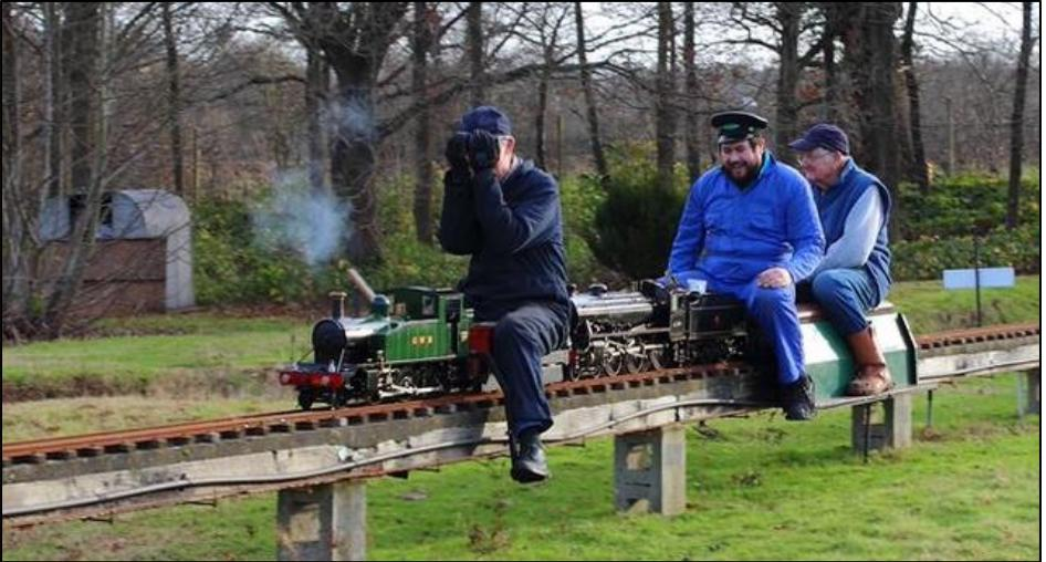
Not everyone had a trouble-free day. The embarrassment of this driver requesting a push is evident in this shot. A good fire and thus steam could not be maintained which was explained later when the spark arrester was removed to reveal the blast pipe nozzle lying in the bottom of the smoke box.
