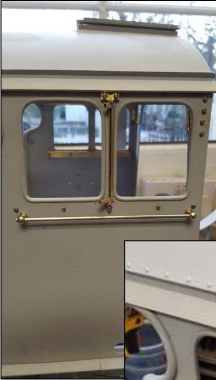
I also machined a semi-circle into the middle of the top bracket so that it was a snug fit up against the single bolt which is where the prototype holds the bracket.
