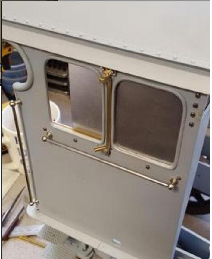
Last picture for this part gives another view of the deflector but also, I have fitted the alloy window templates, leaving the rear slid forward.
