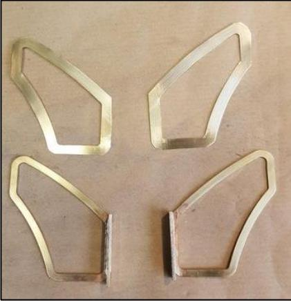
Here we have the frame parts ready, note that the newly cut frames are thicker in section, they are about 0.5 mm deeper where the window sits, the outside edge hasn't been filed to size yet, I'll do that once the glass is fitted.
