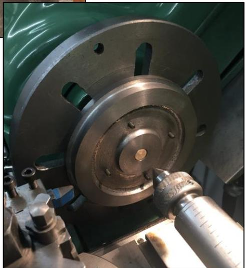
order to ensure concentricity of the bore to the wheel outside diameter I used an old MT2 blank I had in the headstock which I drilled and reamed to take a brass sacrificial plug which I could turn in situ to fit the finished bore of the wheel. I was then able to finish off all of the wheels in the knowledge that they would all be the same
