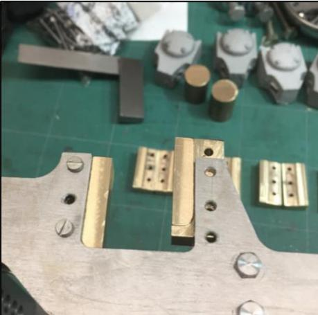
decide to make these from SAE 660 bronze which has the benefit of being good for bearing surfaces and relatively easy to machine. I could only get this in round bar but it machined well with the use of cutting oil. I machined four sticks with the right profile, making sure I made a drawing of the modification I had made for future reference if needed, and got four horn guides out of each stick. After drilling the holes and filing the radius to suit the bogie frame I trial fitted these.
