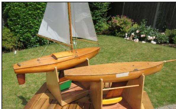
very tatty sails, but I usually make my own so no problem. Closer inspection showed two lovingly made wooden hulls, both polished and beautifully finished and of bread-and-butter construction. There was a hole for a mast, but how much space was there beneath the deck? I poked my trusty endoscope into the hole and the other end plugged into my laptop turned on the light and looked into the unknown.
