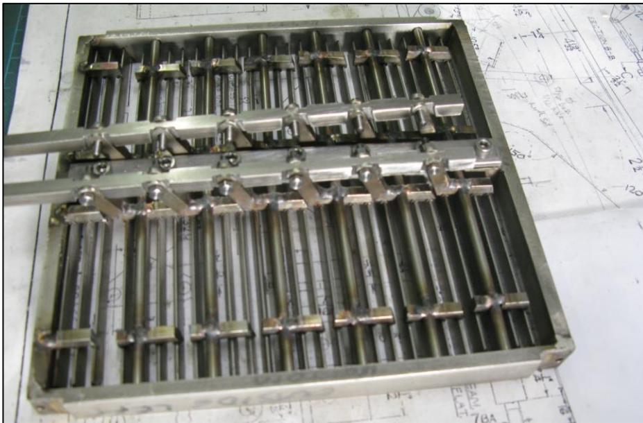
At the moment temporary screws are in place through the clevises and the operating bars have yet to be finished to length. The closing bar for the grate axles can also be seen bolted in place with stainless cap head screws.
