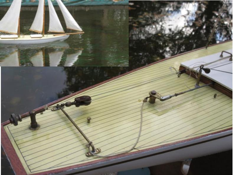
*Stern deck detail note; spring tensioned pulley, the rudder arm is operated by a brass rod from an internal servo.*
