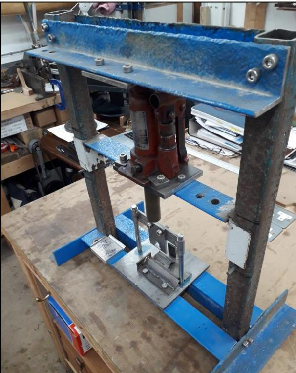
frames have to be bent and to make a tidy job of this I constructed a bottle jack press from an old car jack I had under the bench and the remains of a glider trailer. I also made up a press tool with fence and depth stop so I could ensure repeatability with each bend.
