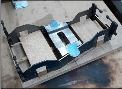
I also made up a smaller press tool so I could bend the side plates that mount on the side of the bogie and contain the lateral spring mechanism.
