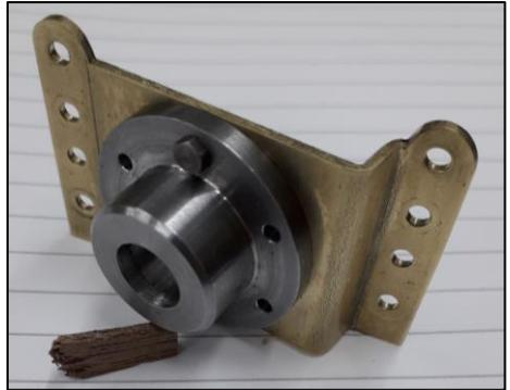
These had to be bent so that the axis of the central hole was perpendicular to the longitudinal axis of the bogie.
