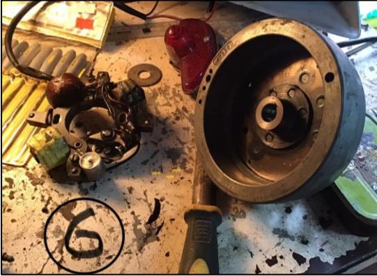
have taken photos of the wheels before the spokes removal to help me install the new. I have cleaned the points, (photos6&7) and on hand spinning the generator flywheel I got a good spark, so it bodes well for starting up. I am now sourcing the paint and the four cables, (clutch, front brake, gearbox and accelerator.) I have already got the two new tyres and inner tubes as the existing ones had
