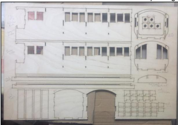
design includes an inner layer of the thicker ply which tabs together with the sides, base and ends to form a solid body. Over this is a spacer layer which allows glazing to be inserted into the middle of the construction. Following this is the outer layer of the coach body which in turn has the beading layer applied. Below are the initial sides with some ends or body profiles.
