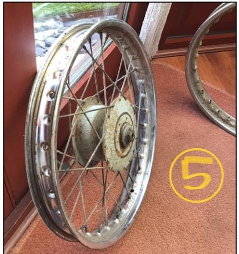
the rusty spokes out of the wheels, (photo 5) I made sure I could buy the new ones as their removal necessitated in their destruction and I
