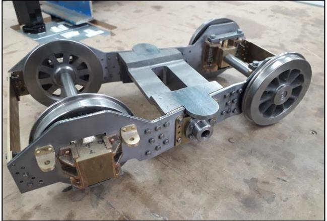
As many will know, the King bogie has the leading wheels on the inside of the frames and the trailing wheels on the outside of the frames. Accordingly, the
