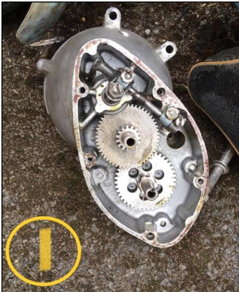
(photo 1) It has two gears, the first is engaged before pulling in the clutch, and the second gear is selected whilst accelerating in first, before pulling the clutch in again to actually change up. As far as I know this worked well. Either Lucas or Wipac Pacy supplied the stator and electrics. With the later models having the luxury of a speedometer that was fitted in the headlamp casing. To stop the engine, you turned off the petrol but obviously
