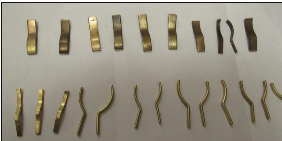
Initially I considered that the way to assemble the coal rails was to silver solder them together, but it quickly became apparent that I needed a secure means of holding each part in its desired position as the rails have a mind of their own once any restraints were removed and that I couldn't silver solder in situ as I had soft soldered the body of the tender to seal it.
