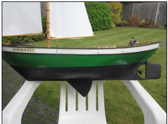
section of the hull. I needed the yacht to turn as easily as possible. Spreading the lead to the extreme ends would give a dumbbell effect and an increased resistance to turning. She weighs in at just over 12 lbs, 5.5 kg. A full catch indeed!
