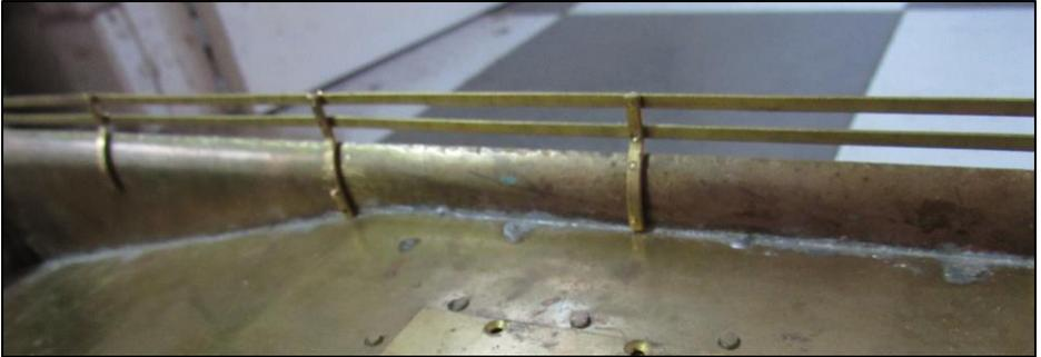
Once the upper rail was aligned and attached it was easier to do the lower rail and at the front this just attaches to the upper rail. **Photo 10** shows both coal rails in place. When I came to make the backing plates, I found that the gaps between the uprights were all very slightly different, so I had to make individual backing plates to suit each and when I was soldering them in position be extra careful to get each one in the right place.
