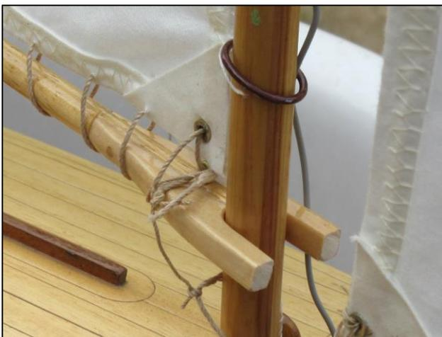
The bowsprit (as per plan) is in hindsight a bit fragile and has broken twice, a hazard when contacting the bank. There is a lower wire connection to the bow at the water level, where there is a hook, this will take the load of the mast flexing when under way. I made all the hooks myself from stainless steel wire about 0.7mm dia with the aid of some tapered round nose pliers, a must for this kind of work.
