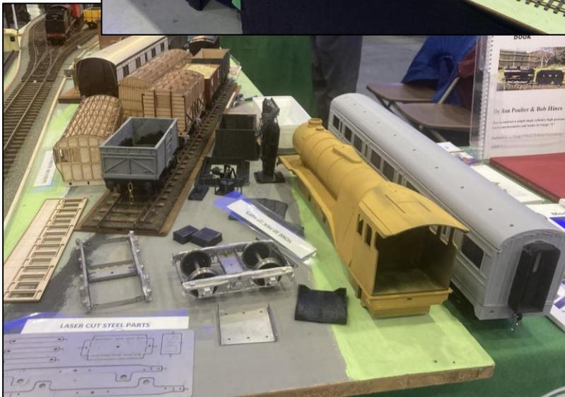
We also featured 3D printed locomotive, coaches, wagons and components, along with laser cut coaches and wagons and metal components.
