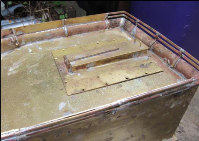
**Photo 11** shows all the coal rails and backing plates in place and soldered into position. There aren't backing plates at the back so the coal rails can be seen more clearly there. There is still a bit of cleaning up to do, but at least I have now completed the coal rails assembly.
