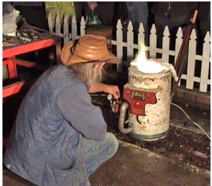
Noel adjusts the gas flow to his air-blown, propane-fired furnace.
