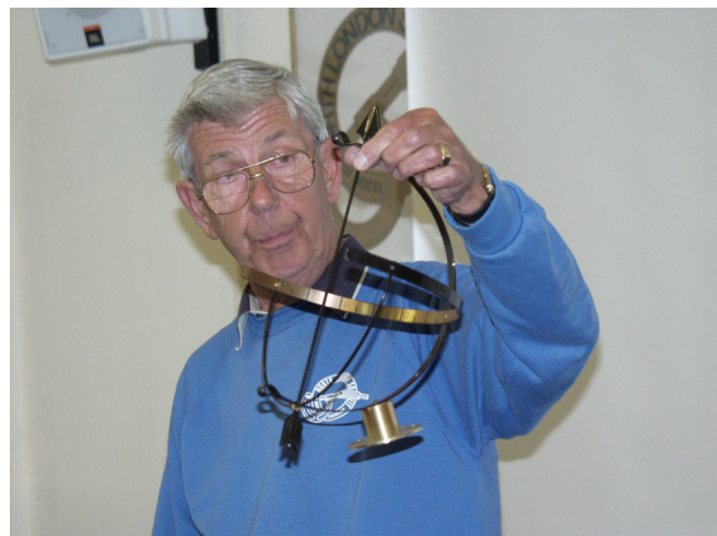
The Mk 2 version; the gnomon is in the form of an arrow, complete with head and fletches, and is made of brass. Photo: Mike Chrisp
