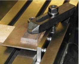
Mike confessed that he would be lost without his table fences. One of a pair is seen here in a table Tslot in use to locate a workpiece for milling. The workpiece registers against the fence and locates against a partly hidden cylindrical stop. A plate clamp and heel block provide the clamping force.
