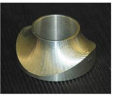
While discussing various types of milling machines. Mike referred to Computer Numerical Control an included this example of  $2^{1}/2$  axis CNC milling of a 5in. gauge Rail
