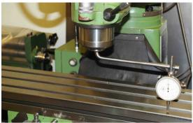
Discussing the alignment of the vertical spindle of a milling machine, Mike showed how a plunger type dial the extent of vertical spindle gauge and L-formed bar is used to sweep from one movement. side of the table to the other. Careful adjustment of the usually hollow with a tapered head brings the dial gauge readings the same each bore at its lower end (nose) into side and sets its axis vertical.
