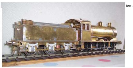
der was built first and the exercise was little different from earlier work in the smaller scales, except that the brass was of thicker gauge. The steel mainframes were drilled and profiled. Machined wheels came from Walsall Model Industries.
