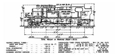
The class that could have been, should have been. Based on Churchward's 3100 series of 1906, engines which worked long lives as Severn Tunnel bankers, Collett increased the boiler pressure from 200 to 225 lb/in<sup>2</sup> while reducing the coupled wheel diameter from 5'-8" to 5'-3" which increased the nominal tractive effort to 31,170 lb; almost as much as the figure attributed to the Castle Class.
