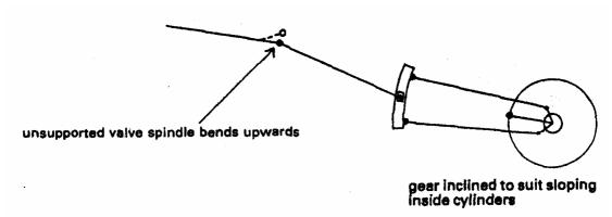
The unsupported valve spindle arrangement on the first 56xx 0-6-2T, showing why it bent upwards
