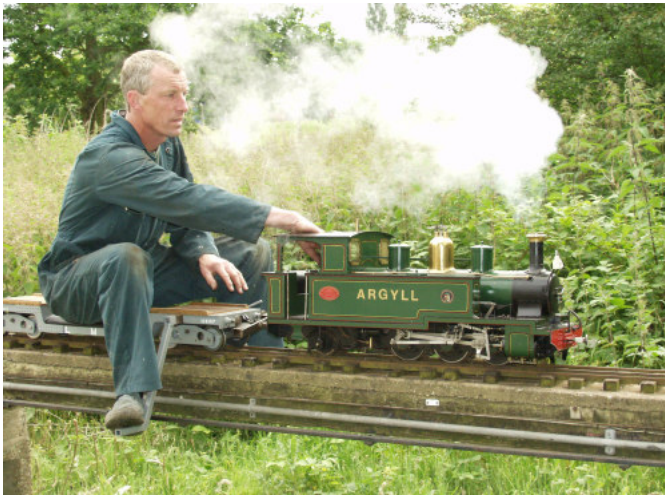
Andy Haresnape's unusual locomotive is fitted with a steel/copper boiler
