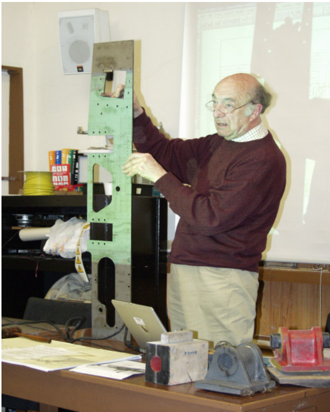
Anna's frames are laser cut; here Derek reveals their size while praising their quality and accuracy.
