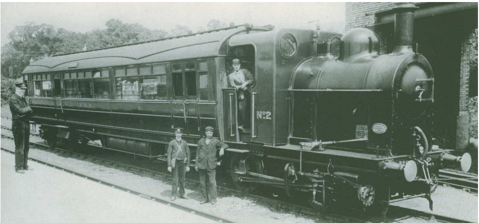
Steam Railmotor No.2, designed by HA Ivatt, seen at Edgware in 1906. The diminutive 0-4-0T mounted on the same frame as the 53-seat car was not powerful enough to draw an extra coach when extra capacity was needed, and was therefore abandoned after about a year.
