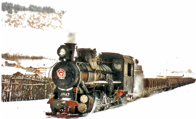
A C2 2-8-2 762mm gauge loco on the Huanan Coal Railway with temp -30C. Photo: Gordon Massey
